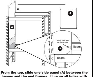
beams and the end frames. Line up all holes with the center of the beams. If the holes are not in-line, the racking beams are incorrectly spaced and will need to be re-adjusted.
