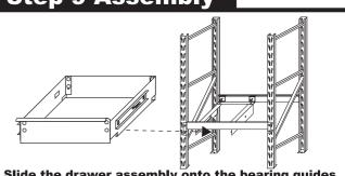
Slide the drawer assembly onto the bearing guides located on the assembled drawer supports. Test to make sure the drawer moves smoothly. If necessary loosen the large screws (G) and large nuts (H) from Step 4 and square up the assembly. Retighten and test the drawer again. Enjoy your new drawer.
