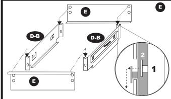
Attach the two drawer fronts (E) to the drawer sides (D-B) by sliding the drawer front (E) tabs into the holes provided on the drawer sides (D-B). Using a rubber mallet, tap on the outside corners of the drawer fronts (E) to secure.
