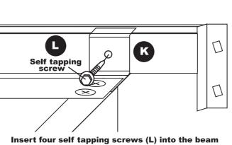
brackets (K). Using a wrench or power drill thread the four self tapping screws into the two racking beams. Tighten the four self tapping screws (L) into racking beam to secure.
