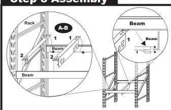
Slide the assembled drawer supports (A-B) onto the inside bottom of the racking beams. Start by sliding the (1) side of (A-B) onto the inside beam edge. Finish by sliding (2) onto the second beam.
