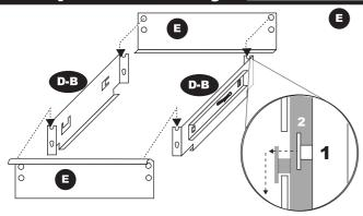
Attach the two drawer fronts (E) to the drawer sides (D-B) by sliding the drawer front (E) tabs into the holes provided on the drawer sides (D-B). Using a rubber mallet tap on the outside corners of the drawer fronts (E) to secure.
