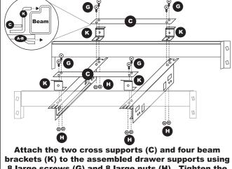
8 large screws (G) and 8 large nuts (H). Tighten the large screws (G) and large nuts (H) securely.
