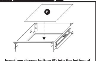
Insert one drawer bottom (F) into the bottom of the drawer assembly.
