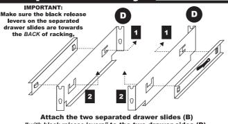
"with black release levers" to the two drawer sides (D). 1, Slide the rear of the drawer slide (1) through the rear slot of the drawe
