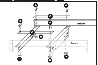
Attach the two cross supports (C) to the assembled drawer supports using 8 large screws (G) and 8 large nuts (H). Tighten the large screws (G) and large nuts (H) securely.
