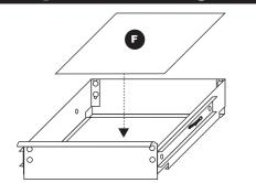
Insert one drawer bottom (F) into the bottom of the drawer assembly.
