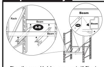
Place the assembled drawer supports (A-B) onto the bottom of the racking beams. This is the position the drawer supports go for a fully boxed beam assembly. Move onto Step 4.
