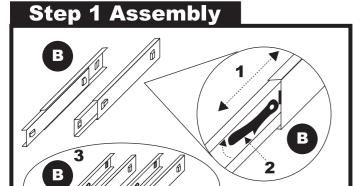
Separate the two drawer slides (B) by sliding each drawer slide (B) apart (1) and while pulling up on the black release lever (2) (located inside each drawer slide) separate the slide. When finished you should have 4 separate sections (3).
